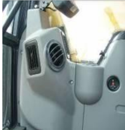
Defrosting vent for front window with better circulation
