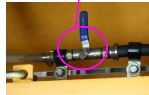
Impurities drainage valve for fuel tank
